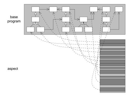
Figure 4.8: Implementing a large-scale feature using an aspect.
