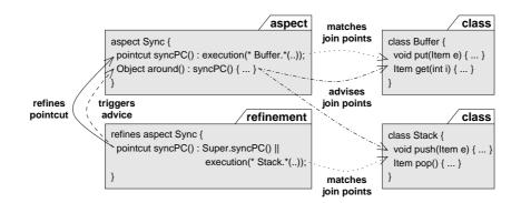
Figure 6.6: The most refined pointcut triggers connected advice.
